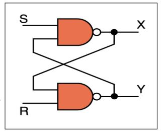
Therefore, if X is 1, the circuit is storing a 1; if X is 0, the circuit is storing a 0
