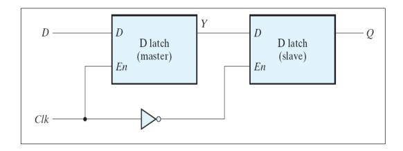
• The change of the D flip-flop output is associated with the negative (positive) edge at the end of the pulse
